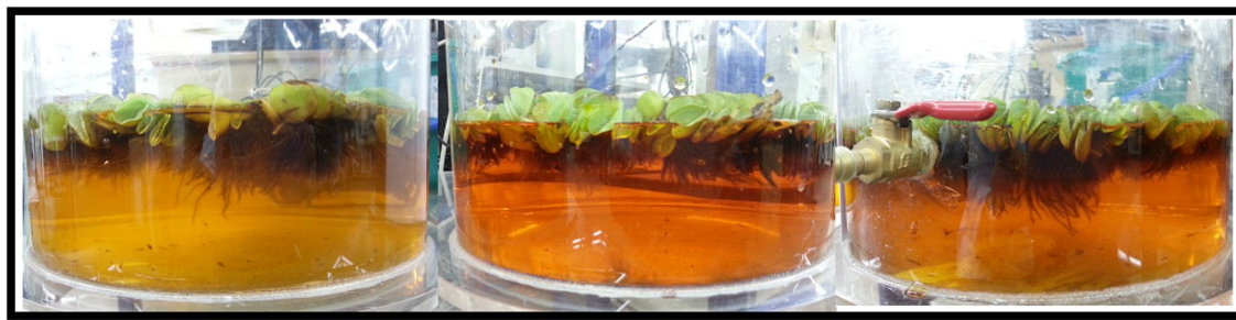
Figure 3. Physical appearance of S. molesta after a 10-day exposure to (a) 5 mg/L MO, (b) 15 mg/L MO, and (c) 25 mg/L MO.
