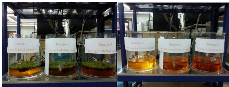
Figure 1. Glass vessel setup for decolorization of methyl orange (MO) (Glass vessel 1 = 5 mg/L MO + S. molesta ; Glass vessel 2 = 15 mg/L MO + S. molesta ; Glass vessel 3 = 25 mg/L MO + S. molesta ; Glass vessel 4 = control glass vessel for 5 mg/L MO; Glass vessel 5 = control glass vessel for 15 mg/L MO; Glass vessel 6 = control glass vessel for 25 mg/L MO).
